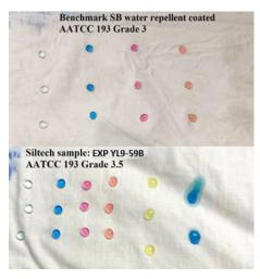
As an alternative to using solvent, various sol-gel systems were prepared with mixtures of **Silmer QT9-30-CG** and several standard silicones and amino silicones. Cotton fabrics were treated and cured in an oven. Water repellency was assessed with AATCC 193 which utilizes dyed solutions of water/ IPA. Results were similar across the sol-gel formulations with contact angles ranging from 110° to 115°.
