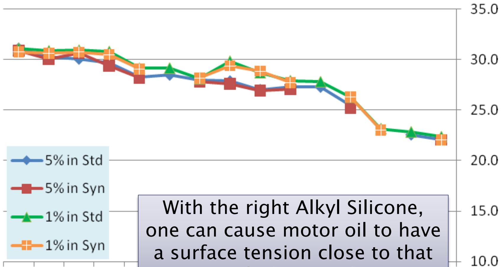
With the right Alkyl Silicone, one can cause motor oil to have a surface tension close to that of silicone oil
