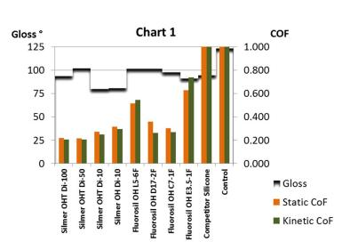
In chart 1, one can see that these products are much better than the control without any additive and the control using 2% of a competitive anti-graffiti silicone, both of which are off of the COF chart scale. Also, **Silmer<sup>®</sup> OHT Di-10** gives the same or more COF reduction than all four fluoroalkyl based **Fluorosil<sup>®</sup>** structures. The slip and properties are also better than those of **Silmer OH Di-10**, a corresponding silicone with different hydroxyalkyl modification.
