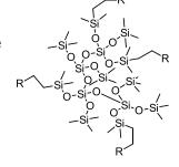
MQ resins are the kinetic reaction products of silicates with trimethyl siloxy groups which generates a silicon-based, cross-linked network having trimethyl silyl functionality on the surface. These types of silicones are often referred to as "MQ resins" because they are built of a network of tetrafunctional silicon atoms (Q group – silicon surrounded by four oxygen groups) end capped with mono functional silicon (M group – silicon with one oxygen group and three alkyls).
