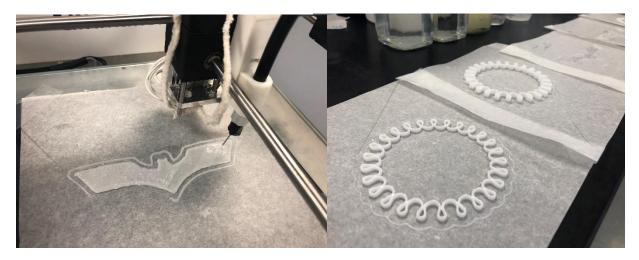
Pictured above right are some bracelets 3D printed in the manner described above. Above left is a bat insignia being printed. The cured resins are opaque white, flexible and reasonably tough.
