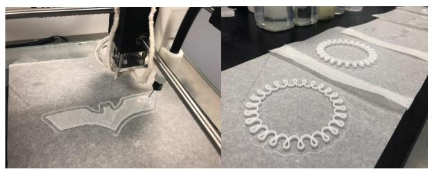
Pictured above right are some bracelets 3D printed in the manner described above. Above left is a bat insignia being printed. The cured resins are opaque white, flexible and reasonably tough.
